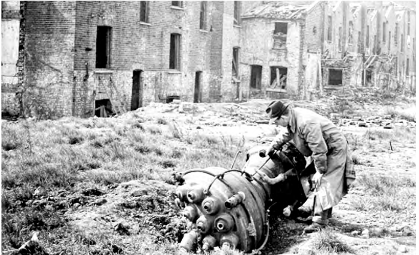
Chinatown (Limehouse, East London) V-2 combustion chamber and venturi which separated from missile on impact. March 1945. http://www.wikiwand.com/en/Limehouse_Causeway
