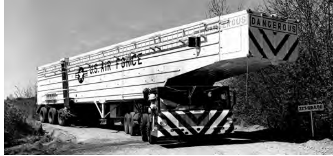
Minuteman missiles are transported overland in a special vehicle called a transporter erector. (Image courtesy of the National Museum of the Air Force)
