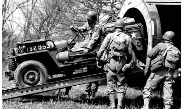
Stripped US Army airborne jeep exiting a Horsa glider, date unknown; note jeep's lack of ends of the front bumper, and some body and fender panels.
